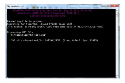
vii. Once the FleaFPGA flash program cycle (approximately 20 seconds with or over 2 minutes without a USB hub!) has completed successfully, with a PS/2 keyboard and VGA monitor plugged in you should be able to play video 'pong'! (To play, use Keys 'A' and 'Z' control paddle #1, while Keys 'K' and 'M' control paddle #2).
