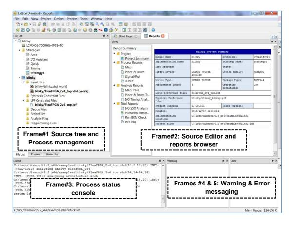
For the remainder of this section, we will be referring to the numbered frames shown above to help emphasize which frame within Lattice Diamond that we're covering.
