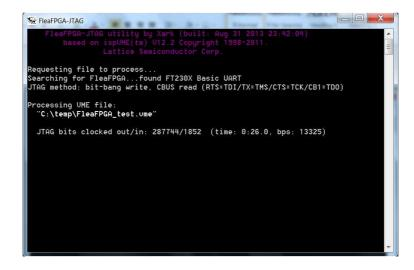
iii. Once the FleaFPGA flash program cycle is complete (and a successful status message appear in the JTAG console window), you should see your FleaFPGA board running the desired firmware. Nothing to it really ☺
